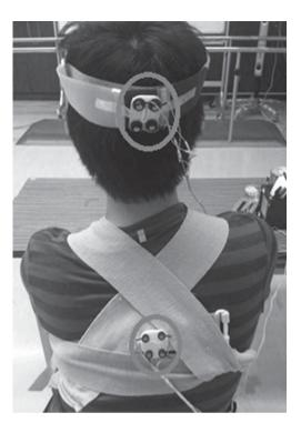
Fig. 4. Two clusters of four infrared light emitting diodes (IREDs) fixed to a rigid surface secured to the participant's head and upper trunk.
