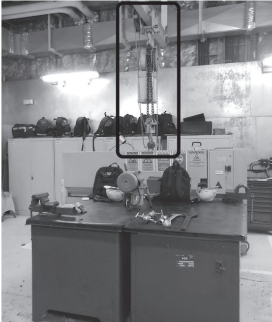
Fig. 4. Disproportionate hoist to the workbench.
