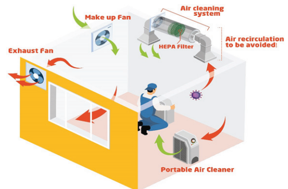
Fig. 2. A schematic view of the proposed engineering controls based on the improvement of ventilation systems.
