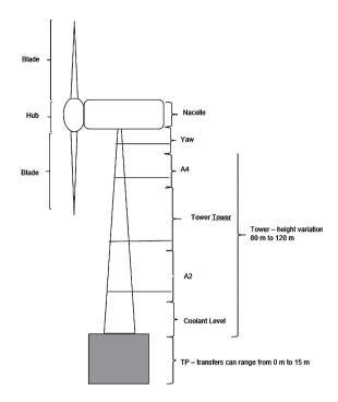
Fig. 1. Schematic of an offshore wind turbine. The schematic is not to scale with variations occurring in all aspects across the industry. The model is based on a 3.6 Offshore Turbine.
