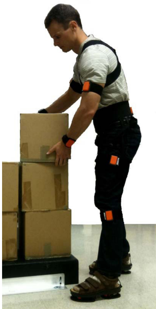
Fig 1. The wearable Xsens measurement system consisting of a full body inertial sensor motion capture system and shoes instrumented with 3D force sensors (ForceShoes). Note that the inertial sensors (the orange sensors) can be worn under the clothes as well.
