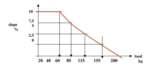
Figure 2 : Limits of load of the garbage container (red line) for different slopes which respects standards requests [2] and RPE = 12.
