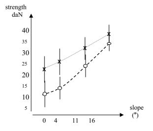
Figure 1: Evolution of average Finit (x) and Fsust (o) pushing forces according to the slope.
