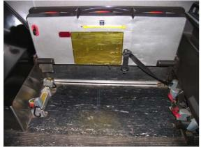
Fig 1: Designated seating area for a WhMD passenger aboard a US bus with the securement equipment (4 tie-downs). Not shown is the occupant restraint.
