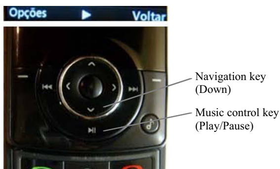
Figure 6. Position of navigation and music control keys on LG mobile phone model
