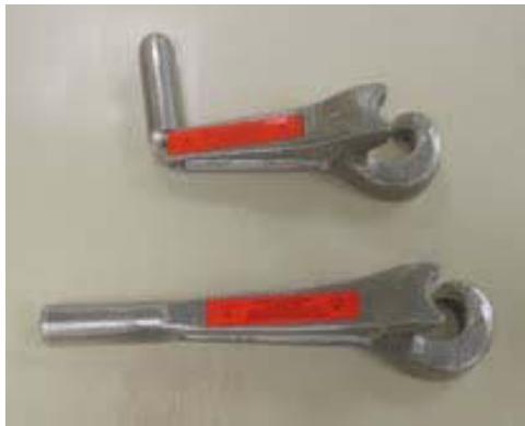
Figure 2. Conventional valve wheel wrench on bottom and modified wrench on top
