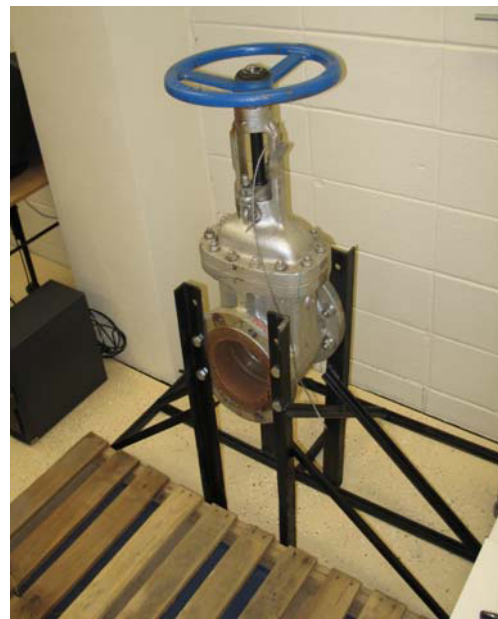
Figure 1. A 6" manual gate valve and a 13" diameter handwheel
