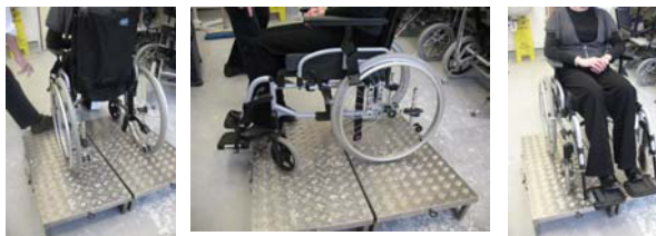
Figure 1. Fixed ramp for checking wheelchair stability
