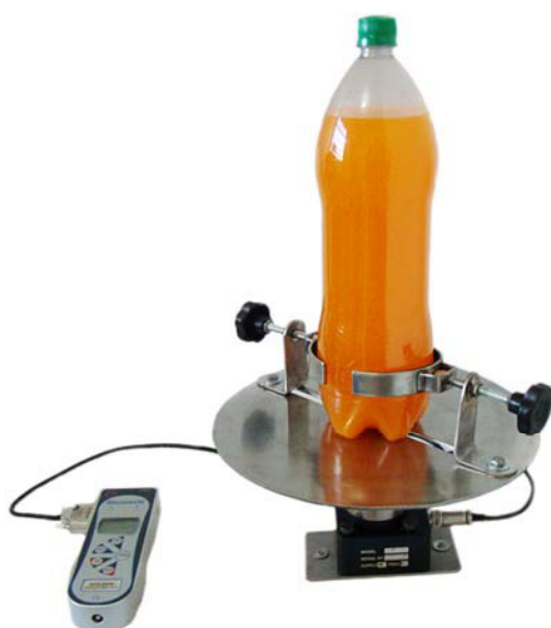
Figure 6. Apparatus to evaluate opening forces of PET bottles.
