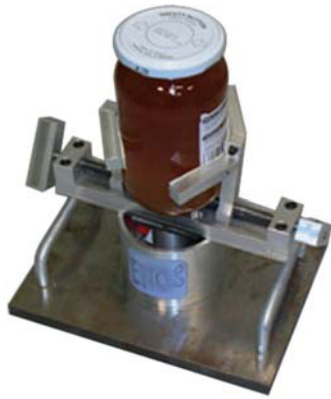
Figure 1. Rig to assess the vacuum jar opening torque [2, p.141].
