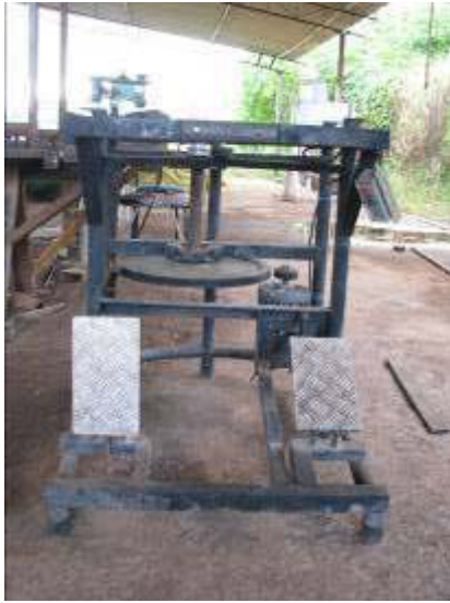
Fig. 8 – Model of the lathe with two pedals, at the finishing phase.
