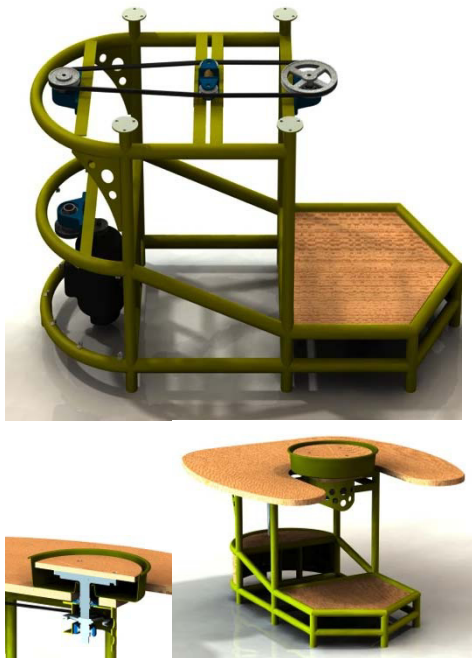
Fig. 3 – Drawing of the transmission system supported by Solid Works .
