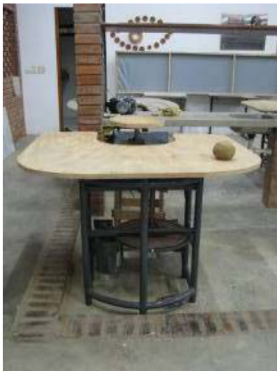
Fig. 9 – Model of the lathe with two pedals, tested by the craftsmen, and already set up in the Architect Wilson Queiroz Campos Júnior Crafts Center.
