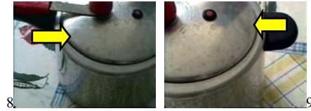
Figures 8 and 9 Images of the pressure cooker - details of the gap in the cover
