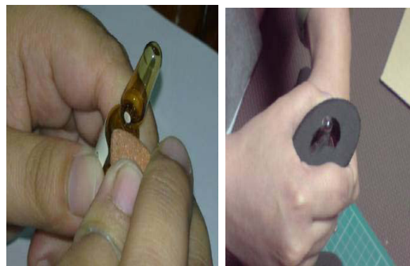
Figure 2 Two methods for snap-off the neck of ampoule
