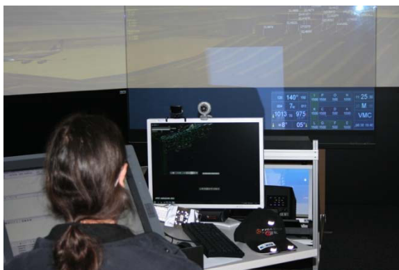
Figure 3 Marker-less head tracker. Tracking works by using a webcam and tracking software
