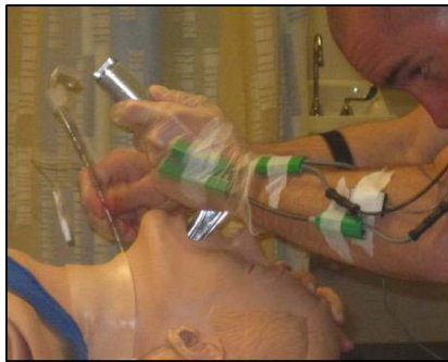
Fig. II – Location of goniometer and torsiometer sensors on left hand and arm
