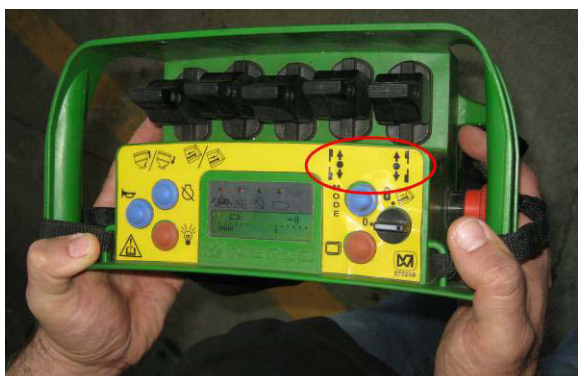
Fig. 2. Portable piloting unit of the compost spreader machine; the circle indicates the icons related to the lever controlling caterpillar tracks movements.
