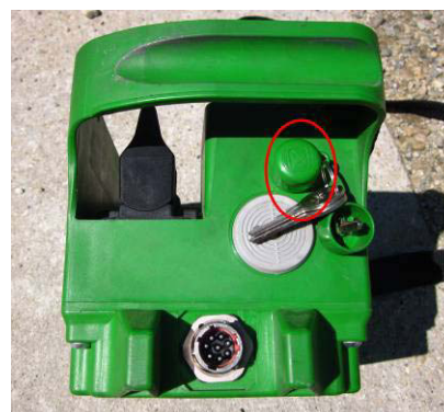
Fig. 3. Portable piloting unit of the compost spreader machine (view from the right side); the circle indicates the key to activate the piloting unit.
