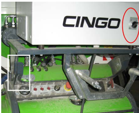
Fig. 4. Detail of teleoperated the compost spreader (view from control side); the circle indicates speed switch, the square indicates the accelerator lever.
