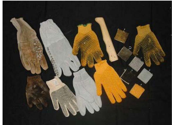
Fig. 2. Gloves, machete handle and specimens used for the determination of the coefficient of static friction.
