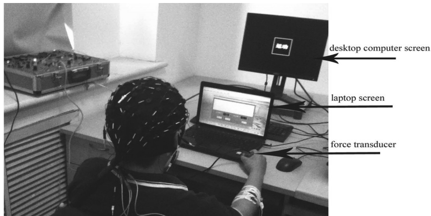
Fig. 1. The desktop computer screen displays the start and end cues of the tasks. The laptop screen displays the handgrip force during the tasks.
