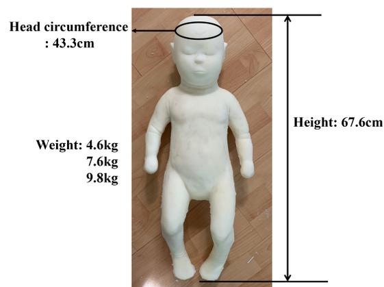
Fig. 2. The specification of the developed infant dummy.
