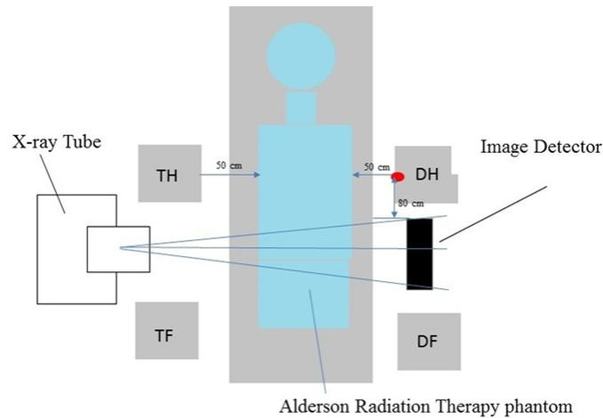
Fig. 2. Scattered radiation experiment using ART phantom.
