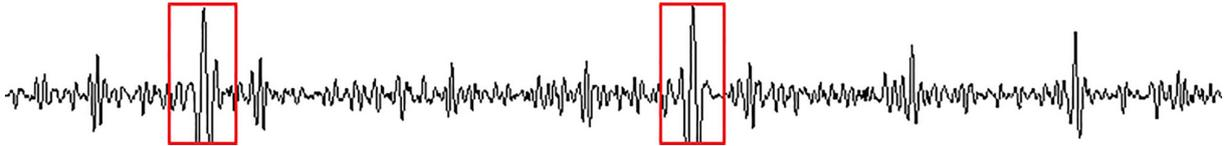
Fig. 6. The separated FCG where the MQRS is misjudged as FQRS (120 bpm).
