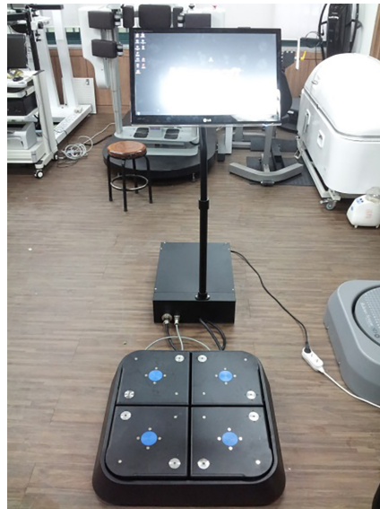
Fig. 1. Quadruple control whole body vibration system for providing exercise load deviation in the left and right side.
