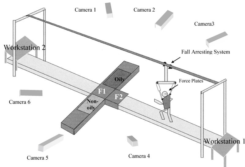
Fig. 1. Field layout of the experiment including Fall Arresting System, Infra-red cameras (6), Linear Slide Floor Changer (LSFC) with force plate (F2) and hidden oily and non-oily test floor surfaces, fixed force plate (F1), and workstations.
