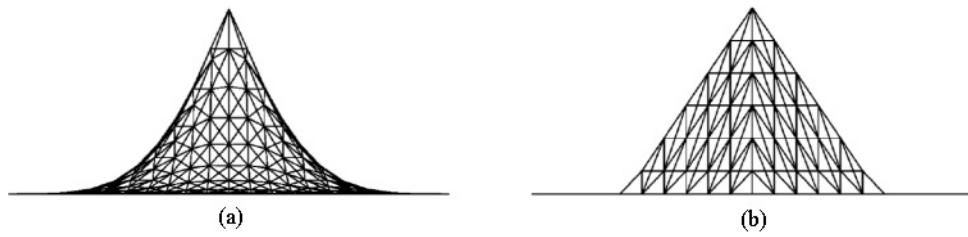
Fig. 4. Deformations of a plane by (a) the proposed CNN and (b) traditional ChainMail method: the deformation produced by the proposed CNN shows nonlinear behaviors whereas it shows only linear behaviors with the traditional ChainMail.
