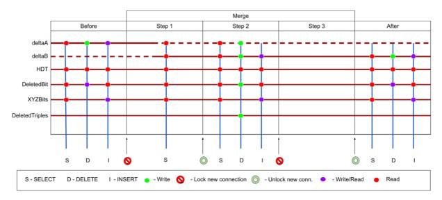
Fig. 2. Figure detailing the merge operation. Horizontally we depict the different merge steps. In each step we detail which operations (SELECT (S), DELETE (D) and INSERT (I)) is possible. Moreover, we vertically depict the data structures that are accessed by the corresponding operation.
