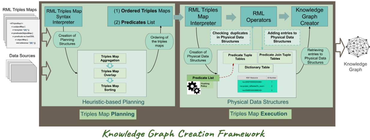
Fig. 3. **The SDM-RDFizer architecture.** SDM-RDFizer receives as an input RML triples maps with its corresponding data sources. The triples map planning component plans and orders the execution of the triples maps. The triples map execution component resorts to physical operators, data structures, and compression techniques to efficiently execute the triples maps in the order stated during planning.
