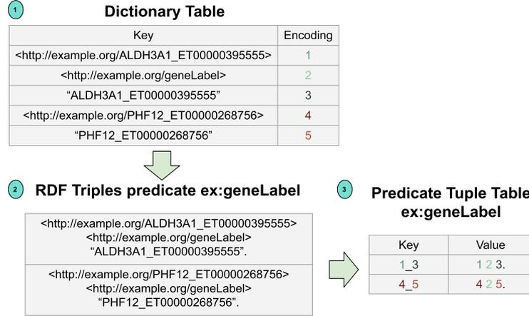
Fig. 5. **Dictionary table and predicate triple table.** Each generated RDF resource or literal is encoded in terms of an identification number in base 36. The dictionary table stores this encoding. RDF triples generated for a predicate, e.g., `ex:geneLabel`, are stored into its corresponding predicate tuple table using the identification number of each RDF resource and literal.
