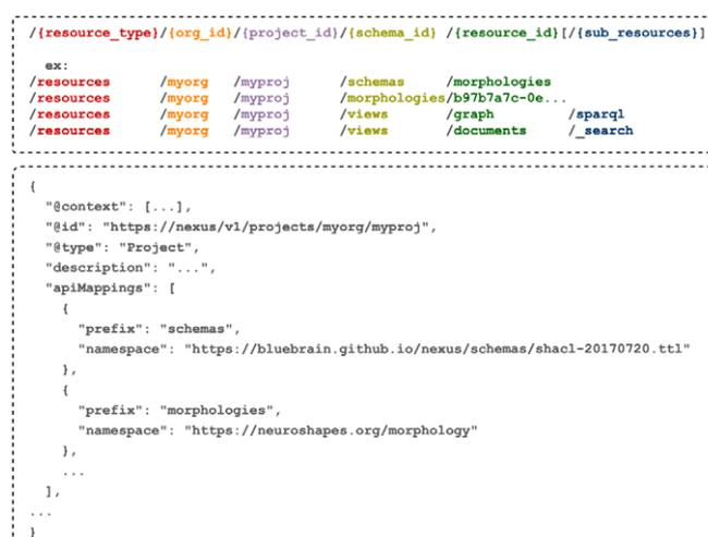
Fig. 8. Resource addressing and identification scheme in Nexus Delta. A project resource can define a collection of aliases and prefix mappings to shorten resource identifiers used in the addressing scheme (e.g. *morphologies* is an alias to “<https://neuroshapes.org/morphology>” and can be used as a segment for identification, either as a schema resource or the collection of resources constrained by it).
