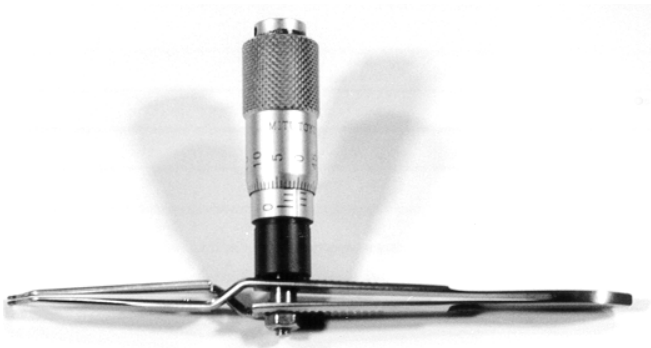
Fig. 3. Crush device used to perform optic nerve injury: This reverse, cross-action forceps produces a mild crush if the tips of the forceps are spaced 0.2 mm apart (in the "closed position") and if the lesion of the optic nerve is made at a 2–3 mm distance to the eye ball (adapted from [113]).
