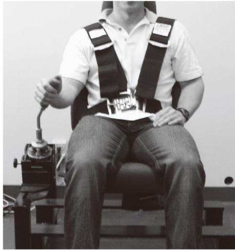
Fig. 1. Participant seated in a laboratory mock-up of an excavator cab.
