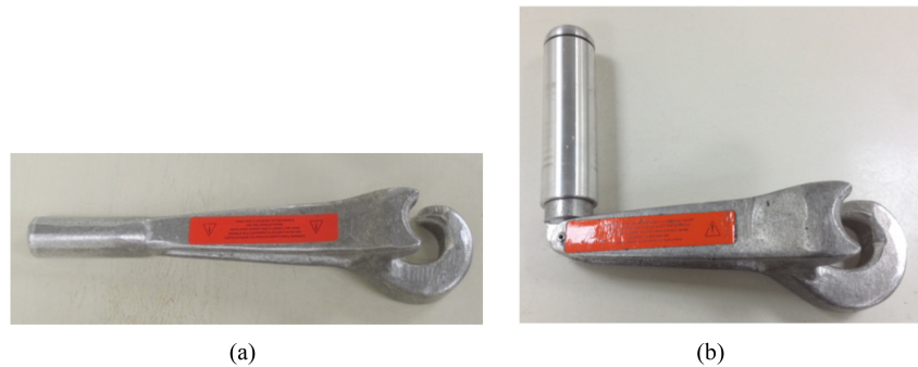
Fig. 2. (a) Conventional valve-wrench; and (b) Ergonomically modified valve-wrench.
