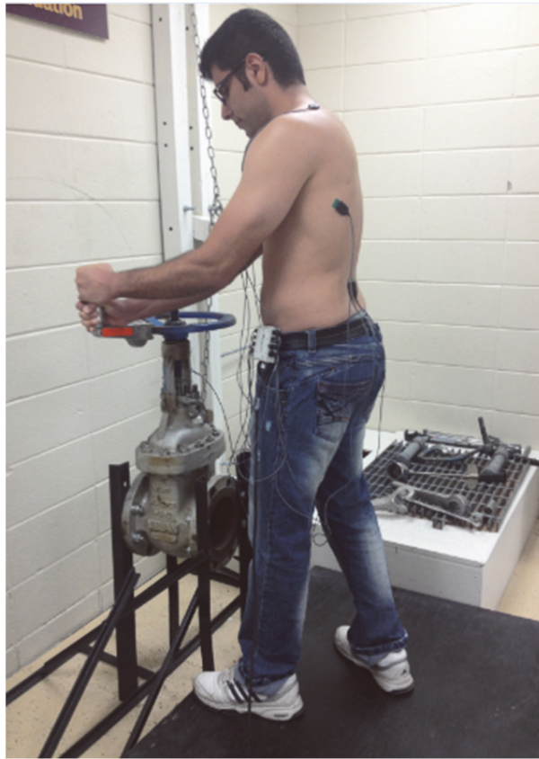
Fig. 1. A 15 cm manual gate valve with a 36 cm diameter handwheel.
