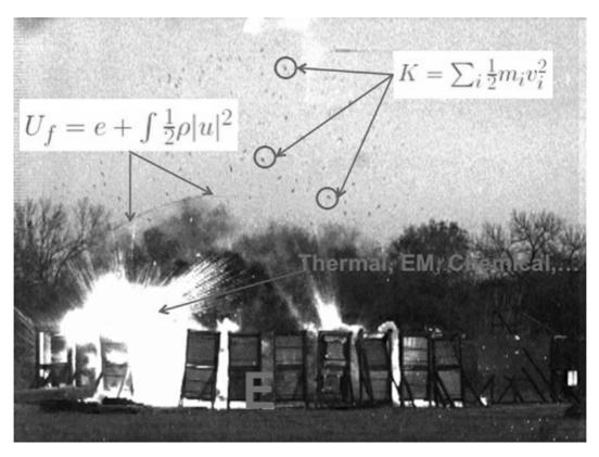
Fig. 1. The total energy conversion from detonation of an explosive charge resulting in kinetic energy of fragments (K), and a shock adiabat  $(U_f)$  together with excess thermal, chemical and electromagnetic pulses (EM). The shock wave and the associated blast wind are responsible for primary blast injury.
