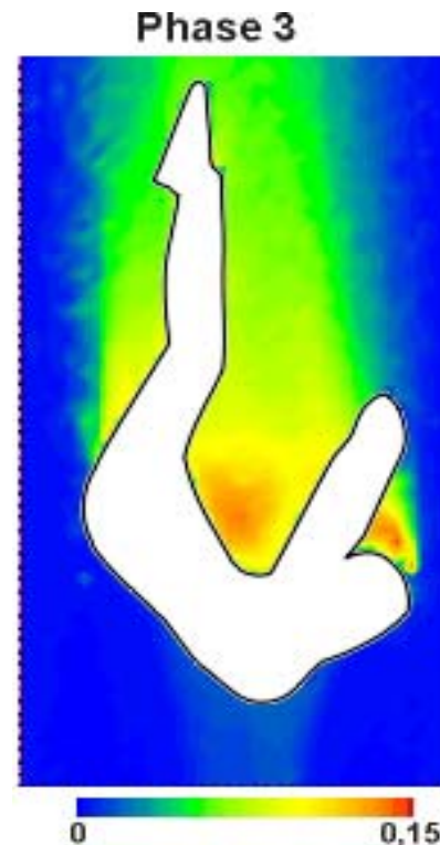
Fig. 2. LDA results of the Reynolds normal stress term u'^2/U_\infty^2 in the cavitation tunnel
