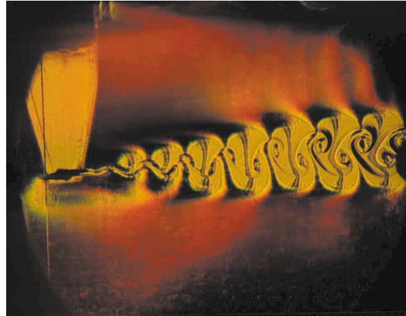
Fig. 2. Weakly stratified brine. Buoyancy period T_b = 17.5 s. Strip is sloped under the angle \alpha = 6^\circ to horizontal and is towed with velocity U = 4.21 cm/s. The asymmetric laminar vortex array is formed from a wavy near wake.
