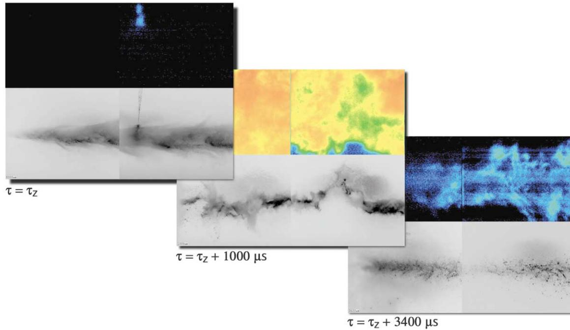
These figures show simultaneously observed images of OH-emission (upper half) and liquid phase distribution (lower half) of near injector region in a cryogenic liquid rocket engine during ignition process initiated by a pulsed Nd:YAG laser. Intensities are shown in logarithmic scales ( $\gamma = 3.3$ ). OH-emission intensities are coded using false colour representation. Images are taken at ignition time ( $\tau_z$ ) and at times 1 ms and 3.4 ms after laser induced ignition.
