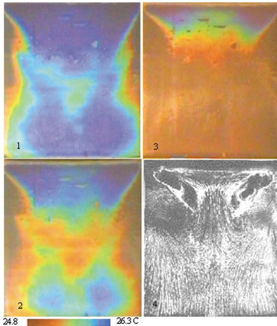
Images (1-3) show a time variation of the surface temperature on lee side of the straight wing obtained by Liquid Crystal Thermography technique. The wing model with symmetric profile and aspect ratio 0.87 was made of wood. The heated model was exposed to the flow and pictures were recorded by a video system. For comparison image 4 shows a flow pattern (limiting streamlines) obtained by liquid film technique (titanium dioxide powder in kerosene).
