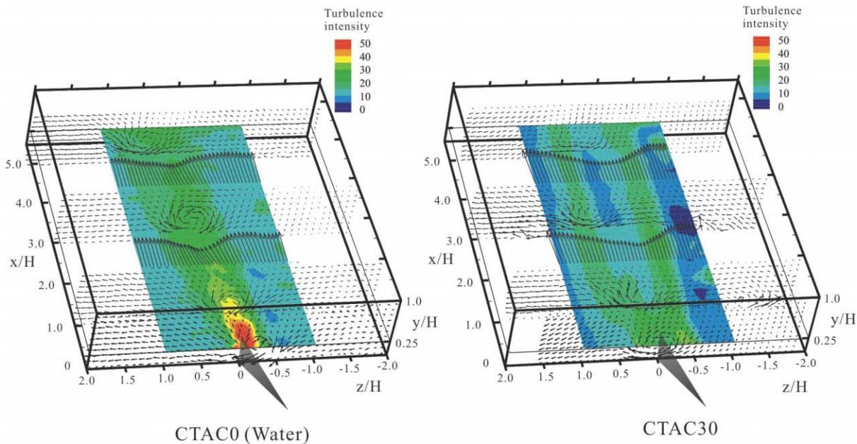
(b) Turbulence intensity distributions and velocity maps of  $(v,w)$ - and  $(u,w)$ -components
