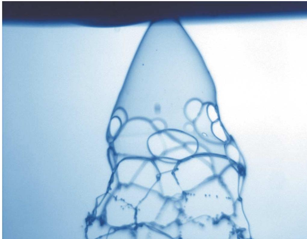
The picture shows the sheet produced by a pressure swirl atomiser at initial stage of break up. The liquid pulverised is a mixture of water and a polymer charge. The liquid is slightly non-Newtonian, and opposite to what occurs with low viscosity liquids, the break up is occurring through the appearance of holes.
