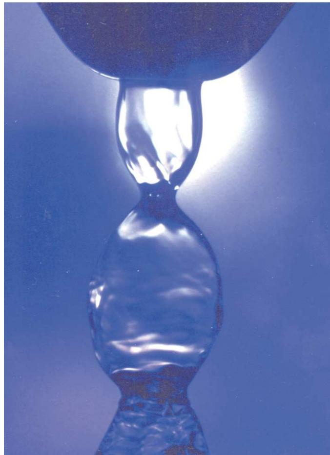
This picture shows the annular liquid sheet produced by a snow generator. This annular sheet is destabilised by a coflowing internal air stream. Different regime of break up may be observed. The longitudinal scales show an encapsulation process. This process was studied extensively and recently modelled at CORIA (X. Jeandel, M. Ledoux. Instability of an Annular Liquid Sheet. The Encapsulation Process. ILASS-EUROPE 2000 Darmstadt 11-13 September 2000)
