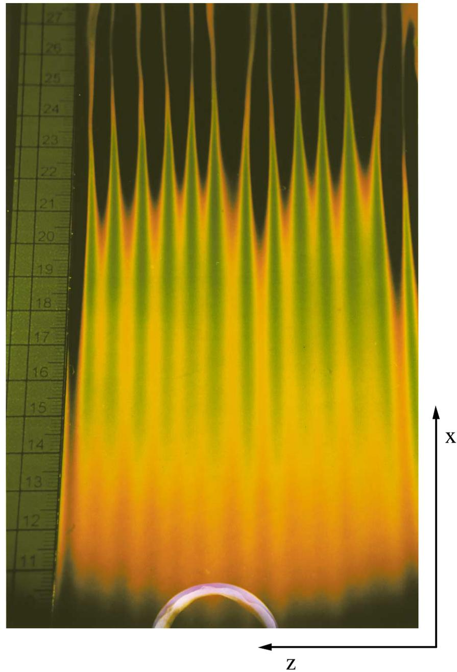
TLC visualization of the surface temperatures of a heated inclined ( $\alpha = 20^\circ$  against the vertical) plate in natural convection. The x direction is the downflow direction. The scale on the left is in centimeters and starts at the beginning of the heated plate. The laminar and longitudinal vortices produce a regular pattern of the surface temperatures in the downflow direction. The TLC change their color with rising temperatures from red to yellow, green and blue.
