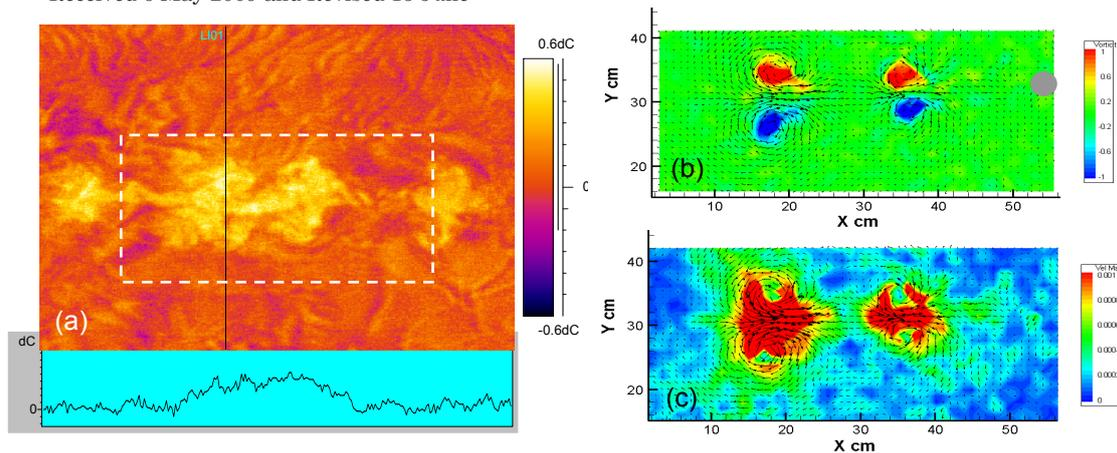
Fig. 1. Thermal (a) and dynamic (b,c) surface signatures of the wake of a submerged sphere [grey circle in (b)] dragged from left to right along the bottom at  $Re=8000$ . In (a) – IR surface temperature (top) and temperature trace along the thin vertical black transect (bottom). In (b,c) - PIV data on near surface vertical vorticity (b) and horizontal velocity (c) inside the dashed area shown in (a).
