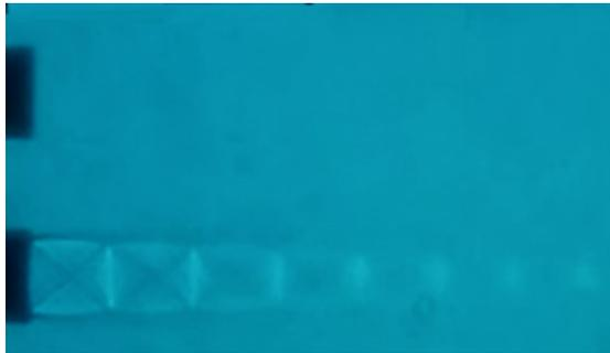
(a) Top nozzle NPR 0, bottom nozzle NPR 3
