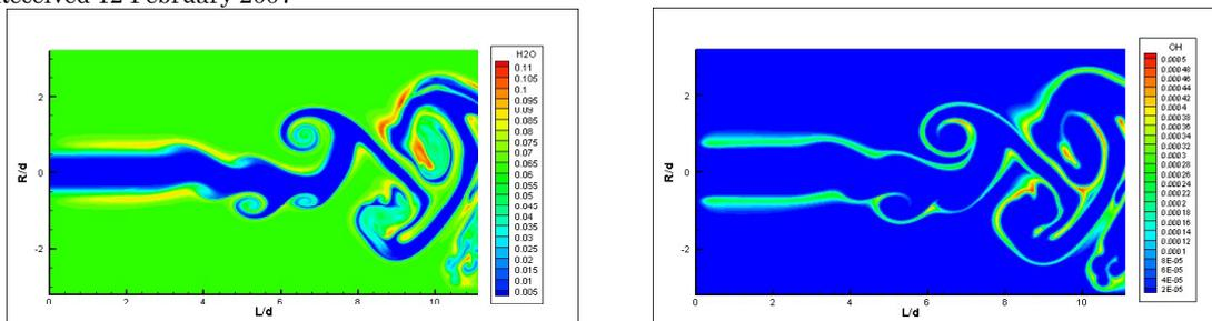
(a) Mass fraction of H<sub>2</sub>O (b) Mass fraction of OH
