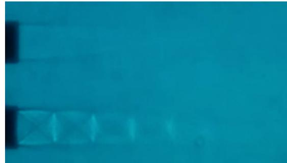
(b) Top nozzle NPR 1.89, bottom nozzle NPR 3
