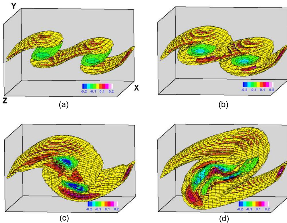
Fig. 2. Three-dimensional profiles of steamwise vorticity with time, (a)  $T = 35$ ; (b)  $T = 45$ ; (c)  $T = 65$ ; (d)  $T = 85$ .
