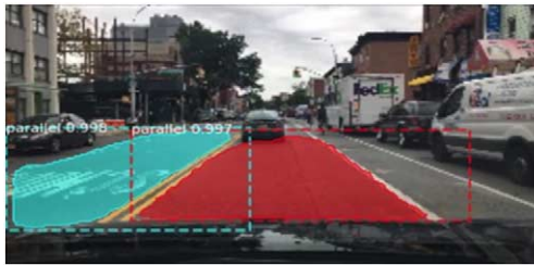
Fig. 12. Lane detection result.
