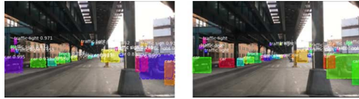
(a) Mask-RCNN prediction result (left) (b) Original image with ground truth label (right)
