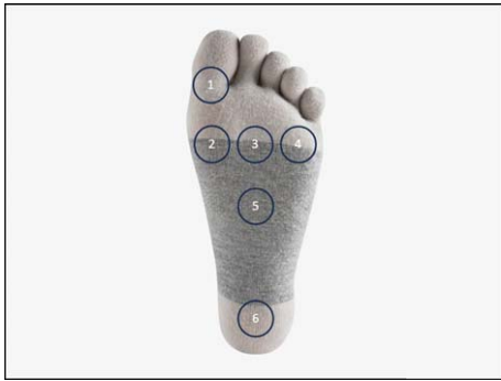
Fig. 1B. Location of Sock Sensors. Bottom of the sock where sensors are placed at the hallux (sensor 1); metatarsal points 1, 3, and 5 (sensors 2–4); midfoot (sensor 5); and heel (sensor 6). More information can be found at https://www.pngkit.com/view/u2e6r5t4q8o0r5w7_bottom-sock-bottom-of-foot-sock/ .
