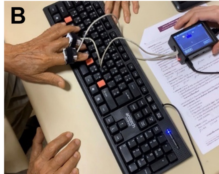
Supplementary Figure 1. The in-house typing kit consisting of a computer program connected to a keyboard (A) and the set-up of the experiment when a participant was asked to type side-by-side alternating between the index and middle fingers on the B/M keys (B).
