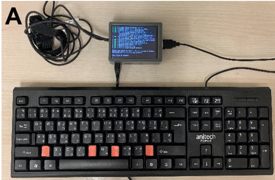
Supplementary Figure 1. The in-house typing kit consisting of a computer program connected to a keyboard (A) and the set-up of the experiment when a participant was asked to type side-by-side alternating between the index and middle fingers on the B/M keys (B).
