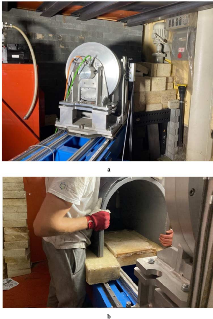
Fig. 239. (A) paraffin blocks shielding (b) shielding on the detector table.
