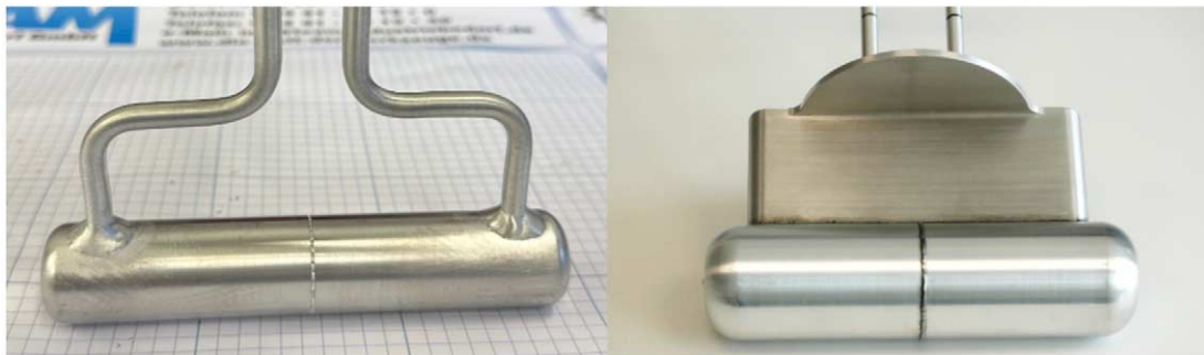
Fig. 230. Manufactured cold moderator (left: hydrogen vessel, right: vacuum jacket).
