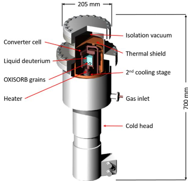
Fig. 2. Scheme of the para-to-ortho converter using the surface contact of liquid deuterium with OXISORB<sup>®</sup> grains. The converter cell is mounted on the 2<sup>nd</sup> cooling stage of the cryo-cooler, while the thermal shield is cooled by the 1<sup>st</sup> stage.
