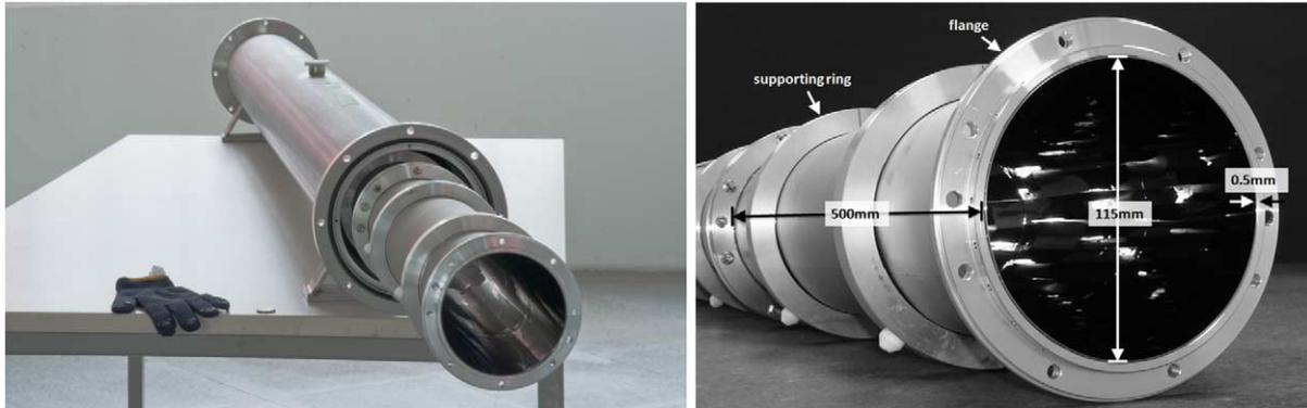
Fig. 5. **Left:** a part of a replica foil with its supporting aluminium ring and its flange at the end of the foil is shown. **Right:** photograph of two connected replica foils with their dimensions.
