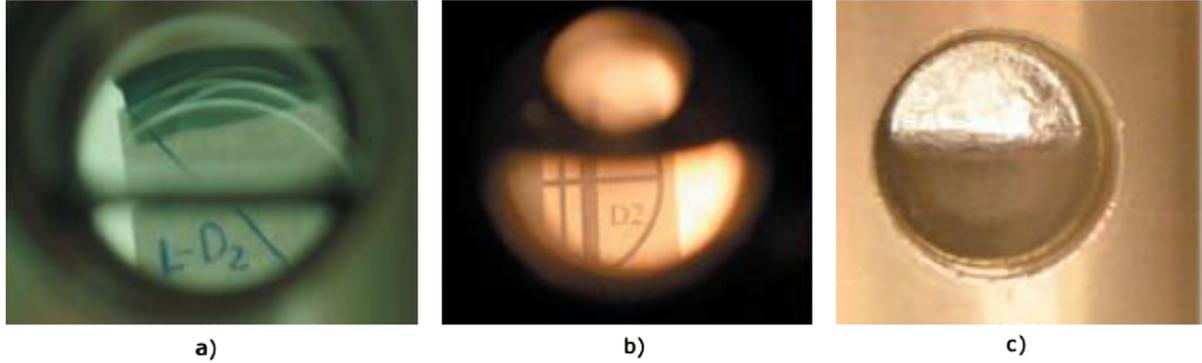
Fig. 3. a) Solid deuterium frozen out from the liquid phase. b) Solid deuterium frozen out via resublimation from the gaseous phase at  $T = 8$  K with an incoming gas flow of  $\dot{V} \leq 30$  sccm. c) Solid deuterium frozen out via resublimation from the gaseous phase at  $T = 11$  K with an incoming gas flow of  $\dot{V} \gg 30$  sccm.
