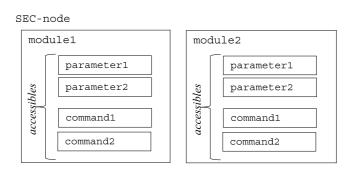
Fig. 2. Schematic illustration of the SECoP structure.
