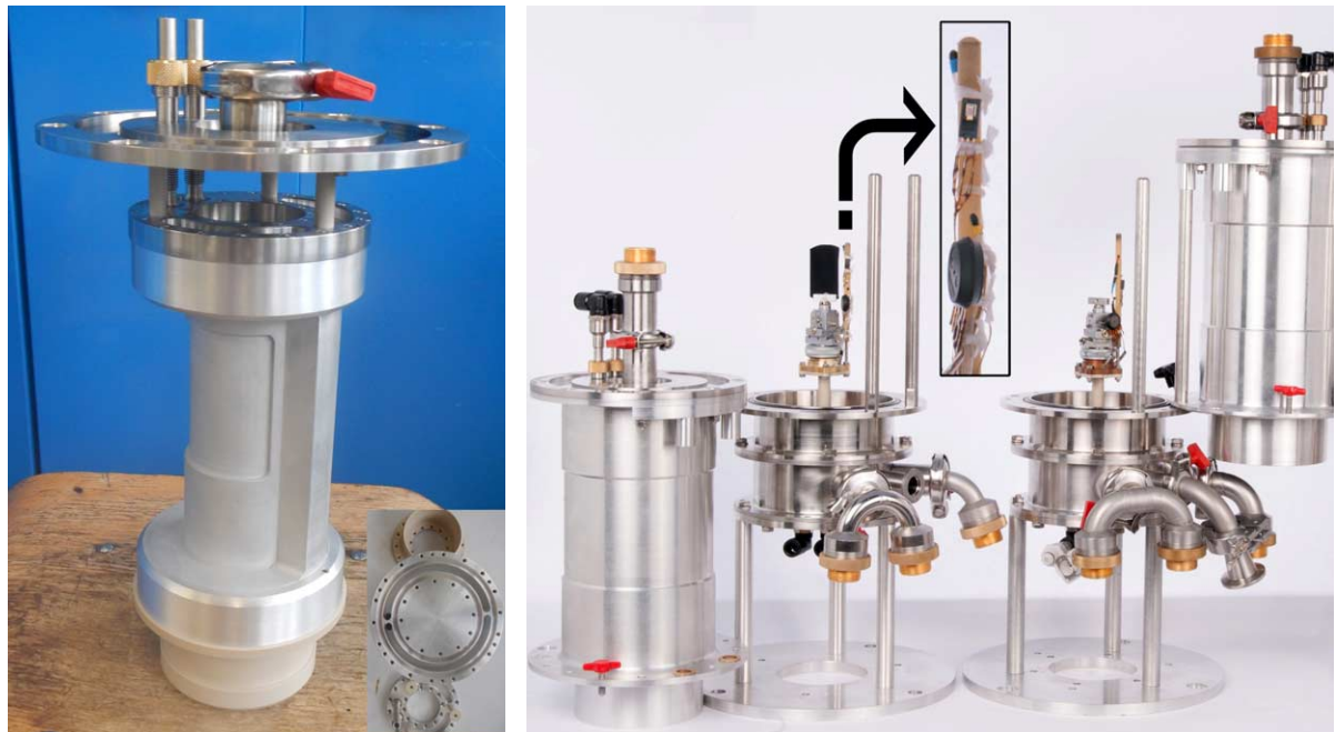
(a) Photo of the assembly of the inner chamber. The insert shows details of the circuitry before assembly. (b) Photos of the lower and upper parts of the humidity chamber. The connectors, the vacuum port and the guiding posts are gathered in the dark angle of the cell.
