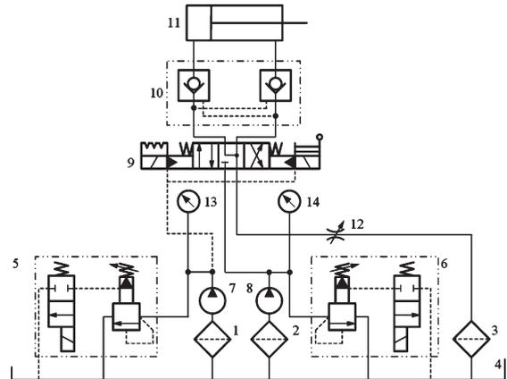
Fig. 7. Principal diagram of hydraulic height adjustment system.
