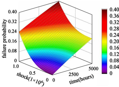
Fig. 9. Failure probability distribution of top event  $y$  without failure correlation.
