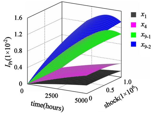
Fig. 10. The first type of probability importance without failure correlation.
