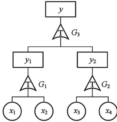
Fig. 4. Multi-dimensional T-S dynamic fault tree for hydraulic system.
