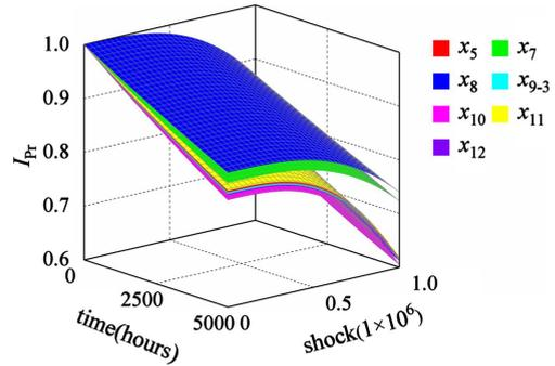
Fig. 11. The second type of probability importance without failure correlation.
