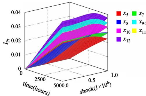
Fig. 18. The difference between the second type probability importance distributions with and without failure correlation.
