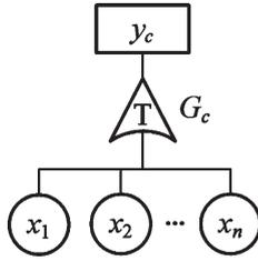
Fig. 6. T-S dynamic fault tree with failure correlation.
