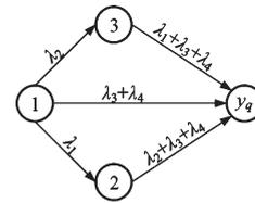
Fig. 3. Markov state transition diagram.
