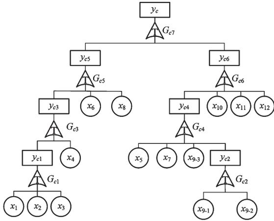
Fig. 12. Multi-dimensional T-S dynamic fault tree copula model for hydraulic height adjustment system.
