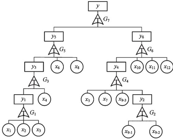
Fig. 8. Multi-dimensional T-S dynamic fault tree for hydraulic height adjustment system.
