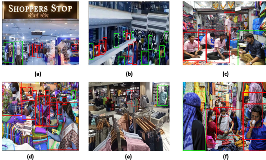
Fig. 13. Measuring the social-distancing through the developed model.
