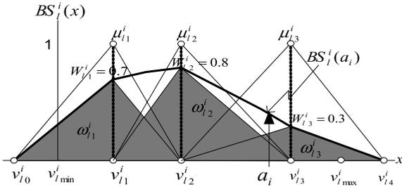
Fig. 3. Structure of bounded sum of three weighted fuzzy membership functions.
